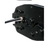
The 75 amp cavity can be used with 50 and 75 amp Powerpole terminals with wire 10 to 6 AWG. That cavity will also crimp many large 'closed' terminals.
